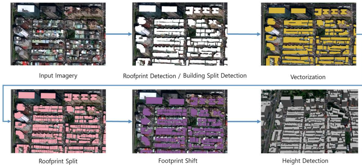
Figure 2-2: Extraction steps of building features
